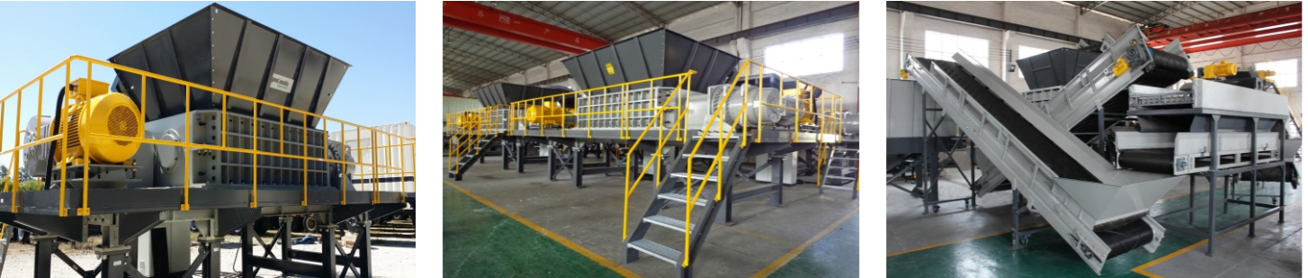
Pre-Shredder 1 Secondary Shredder 2 Return System 3
